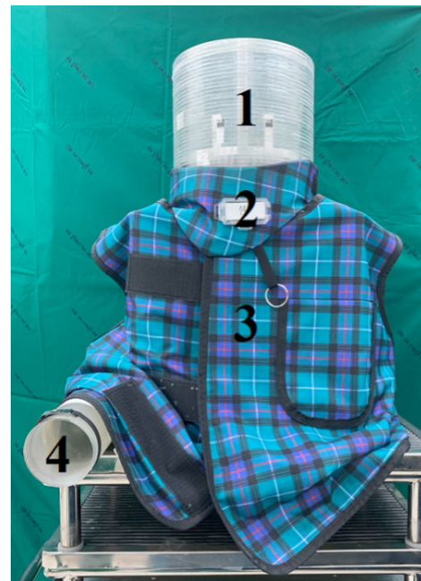
1. eye 2. thyroid (outside the thyroid shield) 3. chest (one is outside the vest and the other is under the vest) 4. wrist
